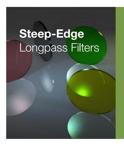
Our steep-edge long pass filters employ magnetron sputtered hard oxide coatings to yield deep rejection and a sharp transition to very high transmission. The coatings are deposited on precision polished Fused Silica substrates, and do not employ any absorbing filter glasses, making them suitable for high-temperature applications. They are offered in three standard sizes, with custom sizes available on request.
