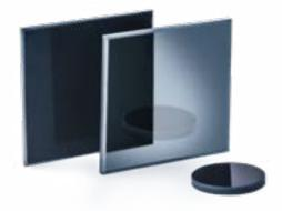
With their ability to minimize back-reflections and scattered light, absorptive neutral density (ND) filters are ideal for calibration. In contrast to the metallic type, absorption-type filters achieve their optical density by absorbing light within the substrate. For this reason, thickness is a key determinant of opacity. Given their absorbing quality, these filters are suitable for low-power applications only.
