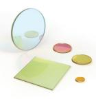
Our steep-edge longpass filters employ magnetron sputtered hard oxide coatings to yield deep rejection and a sharp transition to very high transmission. The coatings are deposited on precision polished fused silica substrates, and do not
